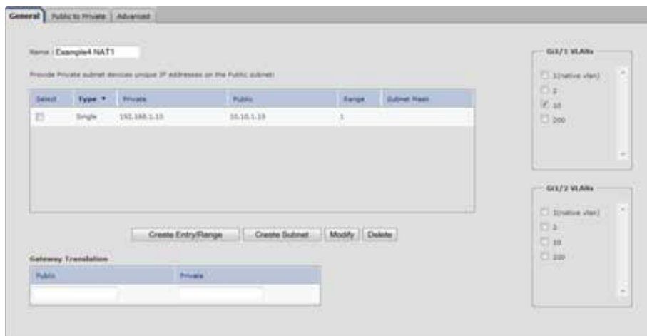
Figure 30 – Machine 1 NAT Switch Configuration (General Tab)
