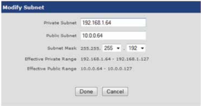
Figure 12 – Example of A Subnet Definition
