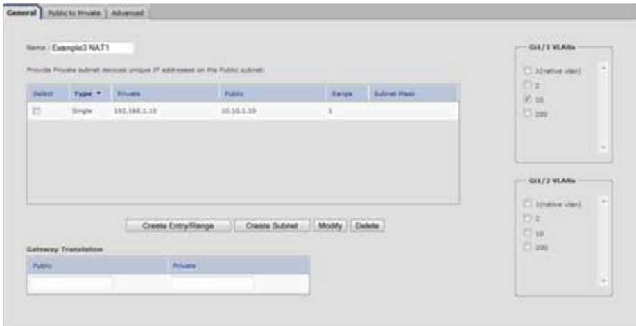
Figure 25 – Machine 1 NAT Switch Configuration (General Tab)
